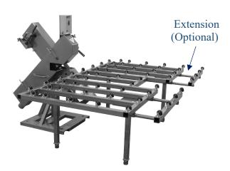
The Twin Seamer Ball Caster Table is specifically designed to work in tandem with a Twin Seamer. The seamer table provides both a cut out for the Twin Seamer machine and Operator. These table cutouts improve operator access during the seaming operation. The ball caster table is suitable for both wet or dry seaming operations; ball casters are chrome plated and subject to minor corrosion over time based on overspray.
